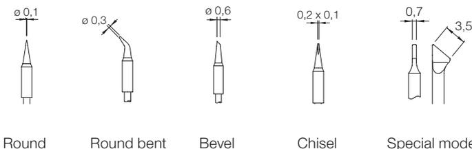
All the cartridges shown are actual size. All measurements are in millimeters (mm). Contact JBC if you need alternative shapes.
