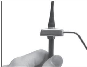
When the tool is in the stand, the temperature falls to 180°C / 360°F (preset sleep temperature).
