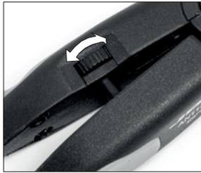
Turn the screw of the tweezers for a vertical alignment of the cartridges. One tip lines up with the other.
