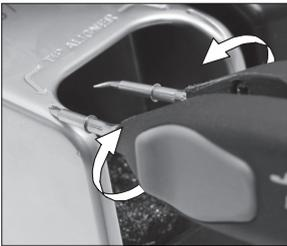
Fit the tip into the aligner and turn to the desired position.
