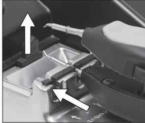
Push the cartridge into the tool to the mark\*.
