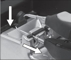
Place the tool in the slot and pull to remove the cartridge.
