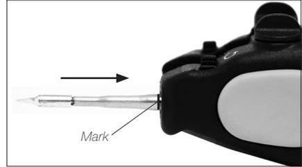
Insert the cartridges as far as the mark for a proper connection. Before inserting, make sure the cartridges are clean to ensure the proper functioning of the tool.
