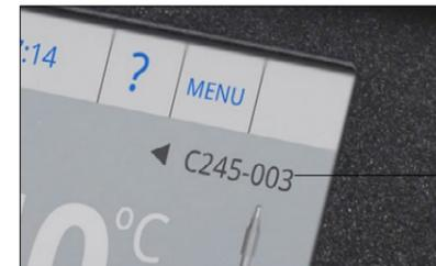
Insert the cartridge model and the station will recognize its characteristics (size and shape) to provide more accurate temperatures
