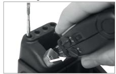
Place the cartridge in the extractor and pull the handle ti remove it
