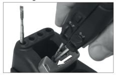
Place the handle on top of the new cartridge and press down.
