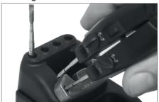
Use the holes to fix the cartridge.
