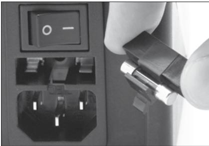
Remove the fuse by pulling the black cap. If necessary use a tool to lever it off.
