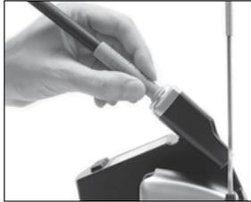
When the tool is in the stand, the temperature reduces to 180°C / 360°F (preset sleep temperature).
