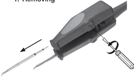
Loosen the screw and remove the cartridge.
