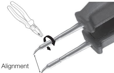
Use a flat pliers for a safe tip alignment.
