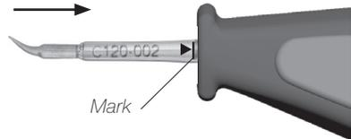
**Important:** Insert the cartridge to the mark for a proper connection.
