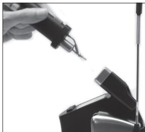
When the tool is lifted from the stand the tip will heat up to the selected temperature.
