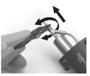
To remove the tip, use a pair of flat-nosed pliers, twist the tip and pull.
