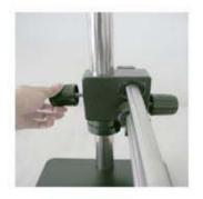
STEP 7 Put the Cap 8 on the top of the vertical post.
