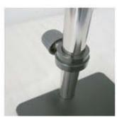
STEP 7 Put the 5/8" adapter in the end of the Dual arm bar.
