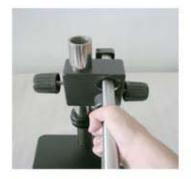
STEP 8 Tight the screw on of the 5/8" adapter
