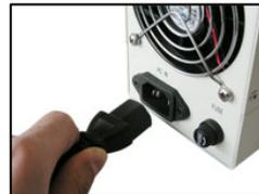
Ensure that the power supply switch is off (downward) and turn the light-adjusting knob anticlockwise to the original position.
