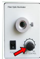
Insert the fiber tie-in into the light-guiding socket and fix it with locking screws.
