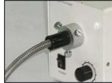
Turn on the power supply switch (upward) and adjust the knob according to the demand.
