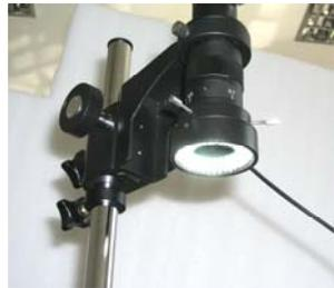
Step 2: Attach the LED light to the microscope.
