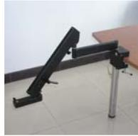
3. The forearm can be adjusted up or down. Please refer to the last step when adjusting the angle.
