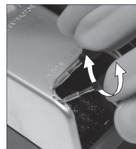
Use the holes to rotate the cartridges for a proper alignment.
