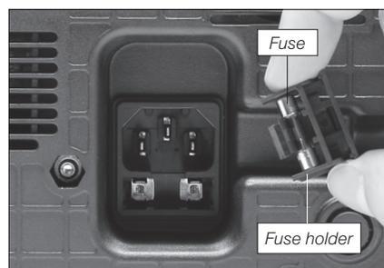
**2.** Press the new fuse into the fuse holder and replace it in the station.
