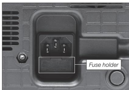
**1.** Pull off the fuse holder and remove the fuse. If necessary use a tool to lever it off.
