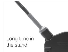
After longer periods of inactivity (pre-set to 30 min.), the power is cut off and the tool cools down to room temperature.
