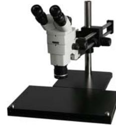
The Hydraulic arm with SZ Zoom Stereo Microscope and
