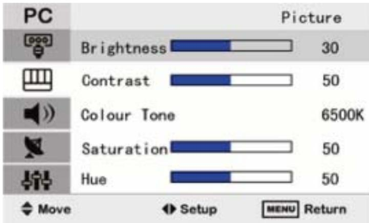
Press the “VOL+” or “VOL-” button, adjust the brightness
