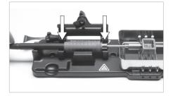
3. Once in place, lock the knob and connect the handle to the stand or the converter (Ref. CHB-A).
