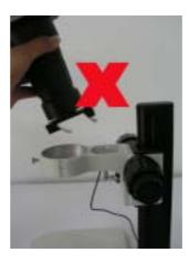
Never put the microscope body with view angle attachment into the scope holder. Before take out the scope body from the scope holder, take off the view angle attachment first.
